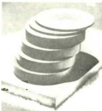
SIX 1.5 IN. DIA. DISKS. FOUR 0.250 IN. AND TWO 0.160 IN. THICK.
